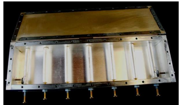
Figure 4 – Inside a cavity filter
