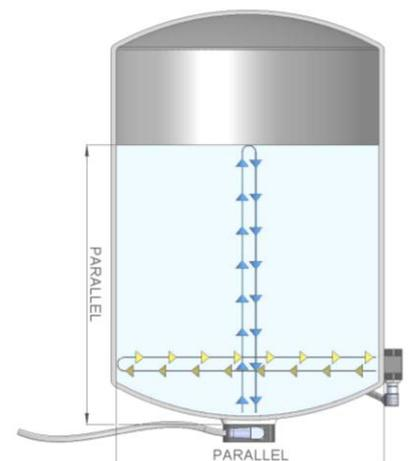
horizontal position. The deviation from horizontal bottom for stainless steel must be less than 10°. Fill the container above half and place the level sensor with silicone in a position expected to be good and calibrate liquid. If there is no error go to **Level Sensor measured data**. The echo strength is shown in dB. Adjust the angle of the level sensor for maximum echo strength. Then calibrate liquid again and check the angle of the level sensor. Then hold it there for 24hours.
