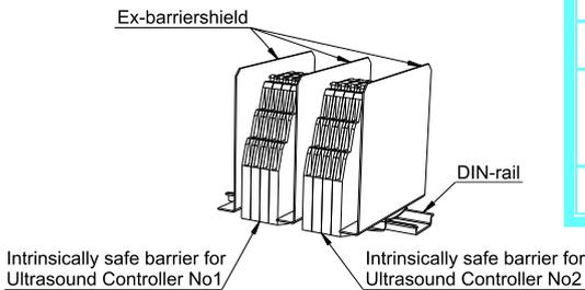
In an ex-installation, shielding aluminum plates must be placed outside each group of zener barriers belonging to each Ultrasound Controller.
