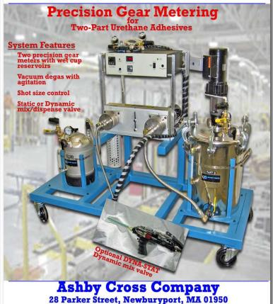
GP80 on a portable cart with 10-gallon and 3-gallon tanks, agitation, and the DYNA-STAT dispense gun
