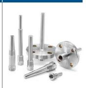
Thermowells are required whenever pressure, velocity or corrosive media exist. Using a thermowell also allows you to remove your temperature instrument without shutting down the process. Standard thermowells are made from solid bar stock, in threaded, flanged or weld configurations. A variety of materials and configurations are available. We offer traceability certifications, wake frequency calculations and a large selection of testing processes to meet all your needs.
