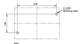
(2) Mounting holes through back of enclosure, accessible with cover removed.
