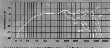
Response contour of Model 2150 measured 15 degrees off-axis. Measured response of a typical production unit does not deviate more than 2.5 dB from the above curve.
