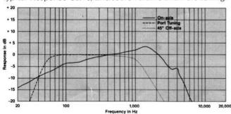
Frequency response of the 2204H in a closed box of 57 L (2 ft³) internal volume. Measured response of a typical production unit, including all peaks and dips, does not deviate more than 2 dB from the above curve. The dashed curve represents the response with a  $160~\rm cm^2~(25~in^2)~port$ ,  $26~\rm cm~(10~in)~long$ , tuning the enclosure to  $50~\rm Hz$ .
