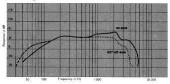
Frequency response contour of the 2220H/J taken in a hemispherical free-field environment, a closed box of 140 L (5 ft³) internal volume enclosing the rear of the driver. Measured response of a typical production unit, including all peaks and dips, does not deviate more than 2 dB from the above curve. The dashed curve represents the response from a  $160 \, \text{cm}^2$  (25 in²) port with a  $13 \, \text{cm}$  (5 in) long duct tuning this enclosure to  $40 \, \text{Hz}$ .
