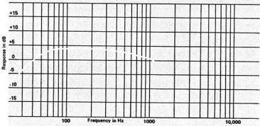
Frequency response contour of Model 2215 in a closed box of six cubic feet internal volume. Measured response of a typical production unit, including all peaks and dips, does not deviate more than 2 dB from the above curve. Additional acoustic loading (passive radiator or port) will further extend bass response.
