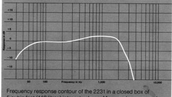
Frequency response contour of the 2231 in a closed box of 5 cubic feet (140 litres) internal volume. Measured response of a typical production unit, including all peaks and dips, does not deviate more than 2 dB from the above curve. Additional acoustic loading (passive radiator or port) will further extend bass response.
