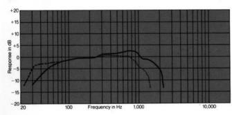
Frequency response contour of the 2240H/G taken in a hemispherical free-field environment, a closed box of 280 I (10 ft³) internal volume enclosing the rear of the driver. Measured response of a typical production unit, including all peaks and dips, does not deviate more than 2 dB from the above curve. The dashed curve represents the response from a  $320\ cm^2\,(50\ in^2)$  port with a  $20\ cm\,(8\ in)$  long duct tuning this enclosure to  $30\ Hz$ .
