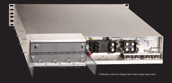
20kW to 30kW Power Supply, 2U x 19" Package, 365VAC to 600VAC, 3¢, Pluggable and Power Factor Corrected, 92% Efficiency at 80% Load Standard Liquid Inlet Temperature is 35°C, 60°C is available 42 to 360 VDC, Ambient Temperature 0°C to + 50°C
