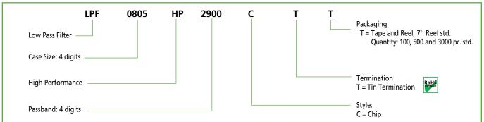
The above part number refers to a Low Pass Filter, (EIA case size 0805), High Performance, Passband DC to 2900 MHz, Chip (C) Style, Tin Termination
