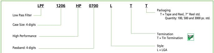
The above part number refers to a Low Pass Filter, (EIA case size 1206), High Performance, Passband DC to 700 MHz, LGA (L) Style, Tin Termination
