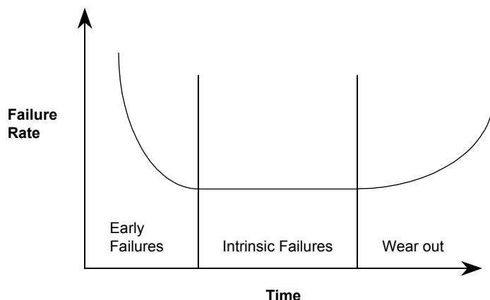
The specific shape and position of the bathtub curve is dependent on the product design, material, processing and defect density for both die and package. When considering the overall reliability of the product, the intended application(s) and the board/system level manufacturing processes will contribute to the observed reliability. As the knowledge and understanding of all these factors grows, designs and processes can be implemented and improved to ensure a robust and reliable product.
