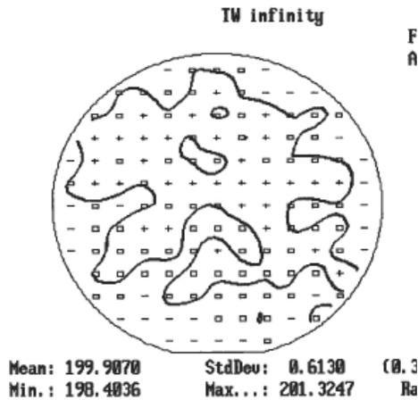
Figure 7: B 5 keV 30 uA unscanned,  $2e11 / \text{cm}^2$ ,  $0.31\% 1\sigma$ , 200 TW units
