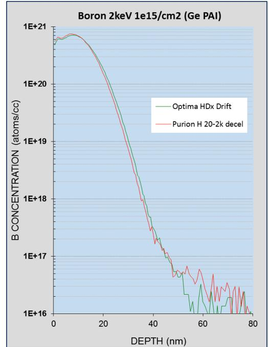
Figure 5: Comparison of SIMS profiles of a reference drift and 10:1 decel implant on Purion H. No energy contamination can be seen on a high-decel Purion H implant at present detection levels of low energy SIMS.
