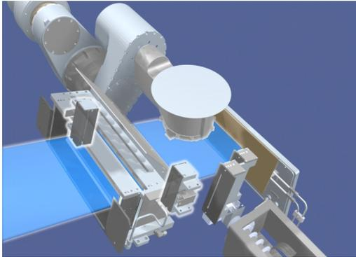
Figure 4: Rendered view of the beam tunnel inside the process chamber. The scanned spot beam is shown in blue, and the microwave PEF is under the beam in close proximity to the wafer plane.
