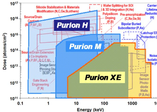
Figure 8: Application space of the Purion platform. Purion H extends the space to low dose, low energy.
