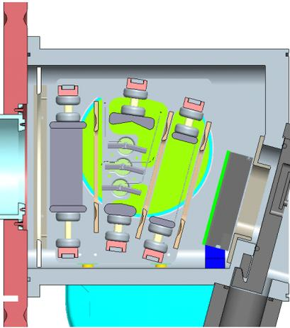
Figure 3: Angular Energy Filter (AEF). From left to right, the optical train comprises: terminal electrode – terminal suppression – decel gap – deflection electrodes – ground suppression. Also shown is a gate valve to isolate the beam line vacuum from the process chamber.
