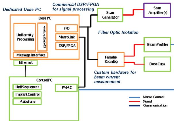
Figure 2: Block diagram of the dosimetry system, including control computers, Faraday interfaces and Faraday cups. Purion H uses magnetic scanning with a single scan amplifier; electric scanning beamlines like Purion M and Xe use two amplifiers.
