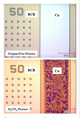
Fig. 10: Optical microscopy of Cu surface after descum showing severe corrosion of Cu after  $O_2/CF_4$  plasma descum in contrast to a corrosion-free surface after  $O_2$ free plasma descum.
