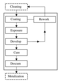
Fig. 7: The process flow diagram which is commonly employed for photosensitive BCB
