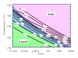
Fig. 4: TTT diagram for Cyclotene<sup>™</sup> polymers.
