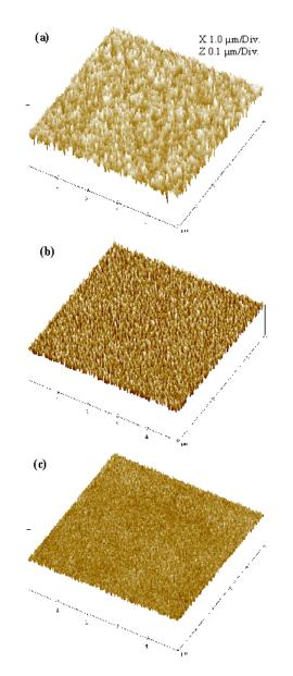
Fig. 11: AFM images of BCB surface after descum. (a): forming gas only; (b): forming gas with 4sccm  $CF_4$ ; and (c)  $O_2/CF_4$ .
