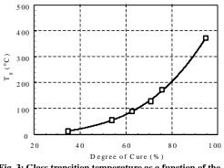
Fig. 3: Glass transition temperature as a function of the degree of cure for Cyclotene™ polymer
