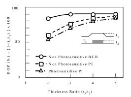
Fig. 6: Degree of planarization for BCB and PI [9].
