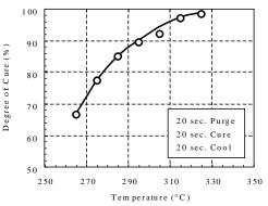
Fig. 5: The degree of cure versus hot-plate temperature for snap curing process for Cyclotene™ polymer.
