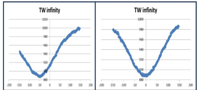
Fig. 7. The TW line-scan values across a wafer implanted from a 300mm GSD at ( $\alpha, \beta$ ) = (0, 4). Wafer map 1 corresponds to -0.3° alpha angle offset before BAC correction, and wafer map 2 corresponds to 0° after BAC correction.
