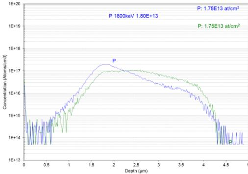
Fig. 6. SIMS dopant profiles of two implants with 0.5° implant angle difference.
