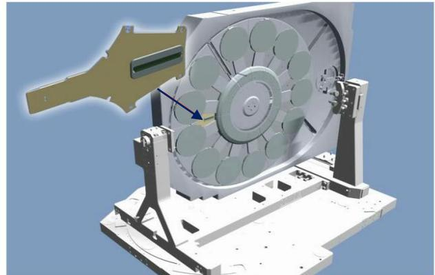
Fig. 3. BAC angle detector mask is located on an inner shield, as depicted in the inset on the upper left corner of this figure of a 300mm GSD disk. The BAC kit delivers beam angle measurement and correction in  $\alpha$  and  $\beta$  directions.
