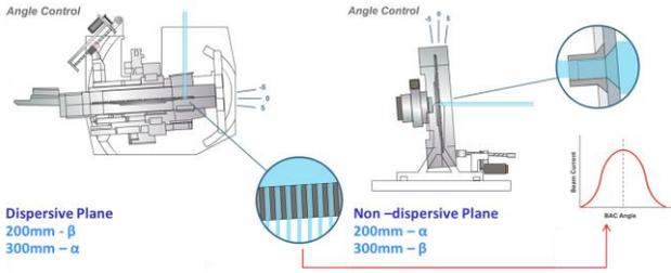
Fig. 5. During the implant start up sequence the gyro will scan from -5.5 to +5.5 degrees in the desired plane while collecting beam current data through the beam angle mask.
