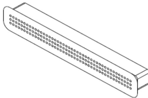
Fig. 4. Beam angle detector mask has 132 holes, which have a 9.6:1 aspect ratio. As the gyro alpha and/or beta position travels over a range of angles provides the data to determine maximum beam transmission.
