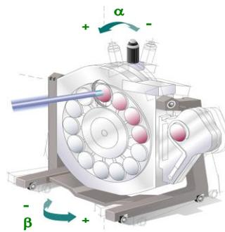
Fig. 1. The GSD end station, showing the orientation of the  $\alpha$  and  $\beta$  tilts.
