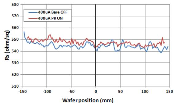
**FIGURE 8.** Vertical Rs linescans of P<sup>++</sup>1800keV 2E13 ions/cm<sup>2</sup> with and without IntelliScan system
