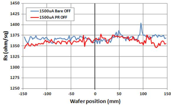
FIGURE 10. Vertical Rs linescans of B<sup>+</sup>1500keV 2E13 ions/cm<sup>2</sup> without IntelliScan system
