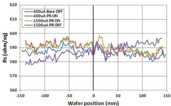
**FIGURE 5.** Horizontal Rs linescans of P<sup>+</sup>770keV 2E13 ions/cm<sup>2</sup> with and without IntelliScan system
