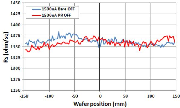
FIGURE 9. Horizontal Rs linescans of B<sup>+</sup>1500keV 2E13 ions/cm<sup>2</sup> without IntelliScan system
