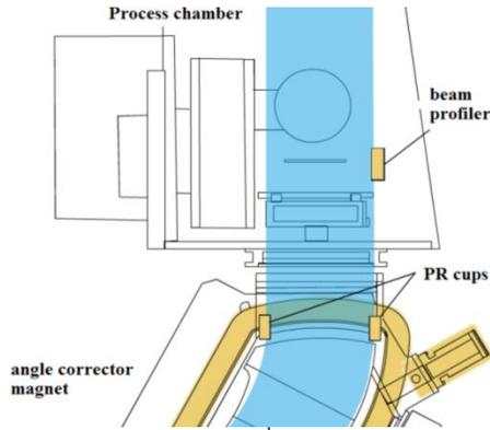
**FIGURE 1.** Layout of 2<sup>nd</sup> half of Optima XEx beam line.
