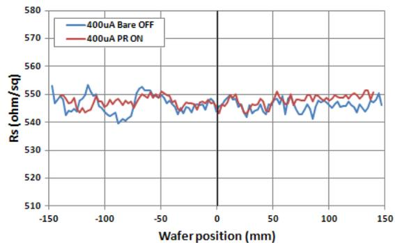
**FIGURE 7.** Horizontal Rs linescans of P<sup>++</sup>1800keV 2E13 ions/cm<sup>2</sup> with and without IntelliScan
