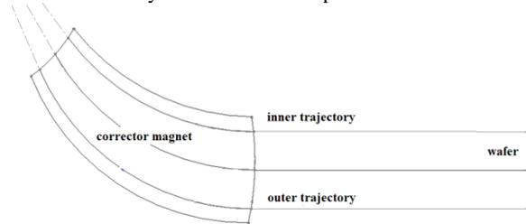
**FIGURE 2.** Beam path length comparison through the corrector magnet on Optima XEx beam line.
