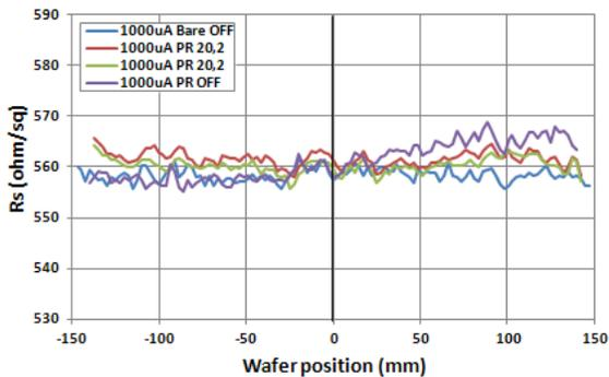
**FIGURE 4.** Vertical Rs linescans of P+1200keV 2E13 ions/cm<sup>2</sup> with and without IntelliScan
