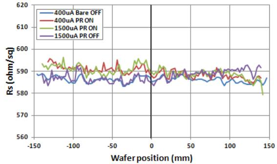
**FIGURE 6.** Vertical Rs linescans of P<sup>+</sup>770keV 2E13 ions/cm<sup>2</sup> with and without IntelliScan
