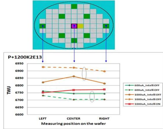
FIGURE 11. Left-Center-Right TW variation of the P<sup>+</sup>1200keV implanted device wafer.
