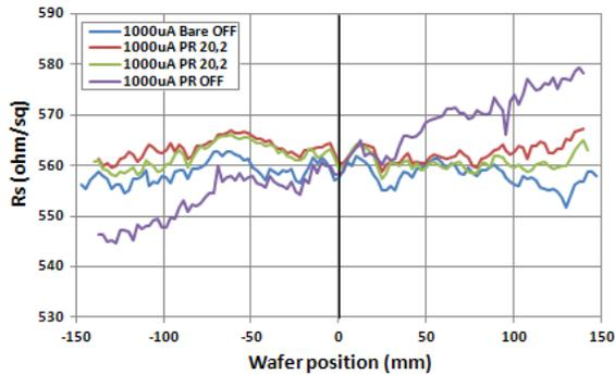
**FIGURE 3.** Horizontal Rs linescans of P+1200keV 2E13 ions/cm<sup>2</sup> with and without IntelliScan system
