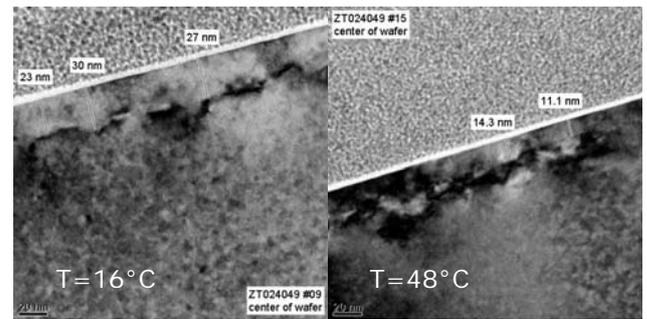
**Fig. 6.** TEM profile of the residuals for 7 keV boron  $5 \times 10^{15}$  cm<sup>-2</sup> implanted on Optima HDx at a wafer cooling temperature of 16°C or 48°C.
