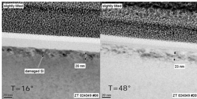
**Fig. 4.** TEM profile of the damage layer below the amorphization layer for 7 keV boron  $5 \times 10^{15}$  cm<sup>-2</sup> implanted on Optima HDx at a wafer cooling temperature of 16°C or 48°C.
