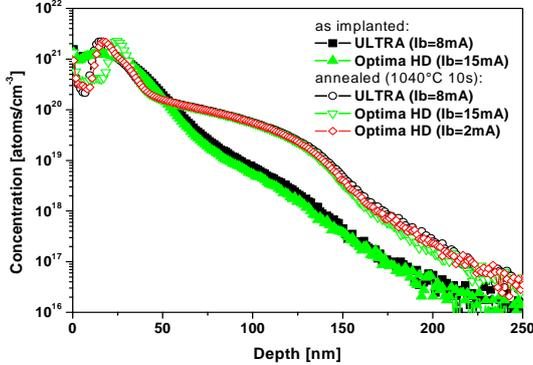
Fig. 1. SIMS profile of  $^{11}\text{B}$  for 7 keV boron  $4.5 \times 10^{15} \text{ cm}^{-2}$  on Optima HDx and ULTRA as implanted and after anneal [4].
