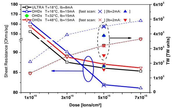
Fig. 2. TW results as implanted and RS results after anneal for 7 keV boron.
