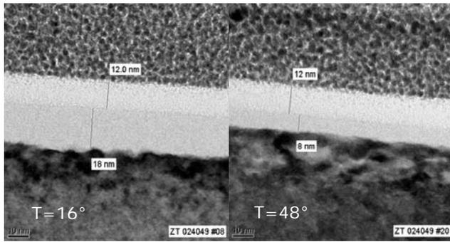
**Fig. 3.** TEM profile of the amorphization layer for 7 keV boron  $5 \times 10^{15}$  cm<sup>-2</sup> implanted on Optima HDx at a wafer cooling temperature of 16°C or 48°C.
