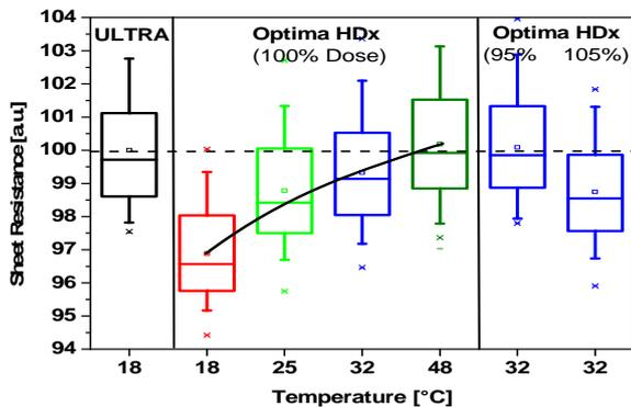
Fig. 7. Sheet resistance results for 7 keV boron  $4.5 \times 10^{15} \text{ cm}^{-2}$  on production wafers (ULTRA and Optima HDx).
