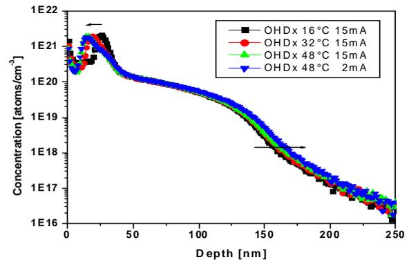
**Fig. 5.** SIMS profile of <sup>11</sup>B for 7 keV boron  $5.0 \times 10^{15}$  cm<sup>-2</sup> on Optima HDx after anneal.
