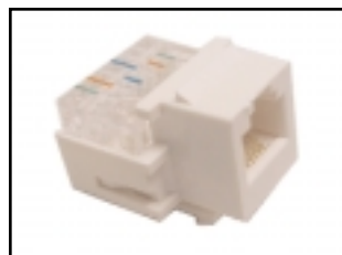
8-POSITION UL KEYSTONE MODULAR JACK IDC type meets level 3 & 4 requirements. 30 microns gold plated contacts and ABS material UL94/A-O. Suitable for 22-26 AWG wire. 72-101-BK..... black 72-101-IV..... ivory 72-101-WH..... white
