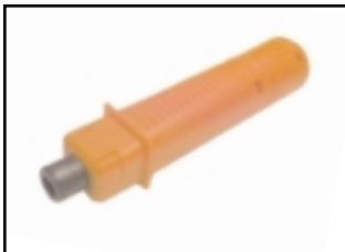
72-234 ADJUSTABLE IMPACT PUNCH DOWN TOOL Provides constant action for seating wire into terminal blocks. Adjustable impact pressure control. The back of the handle is a storage compartment for 1 spare blade. For use with Calrad 72-245, 72-246, 72-247 blades.
