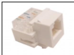
6-POSITION UL KEYSTONE MODULAR JACK IDC type meets level 3 & 4 requirements. 30 microns gold plated contacts and ABS material UL94/A-O. Suitable for 22-26 AWG wire. Will work as a 4 position jack. 72-100-BK..... black 72-100-IV..... ivory 72-100-WH..... white
