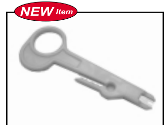
72-239 PLASTIC PUNCH TOOL Inexpensive disposable punch down tool with cable stripping blade for outer PVC jacket. Suitable for small jobs. Works with 5-6mm O.D. UTP/STP cable. Terminates conductors on 110 blocks.
