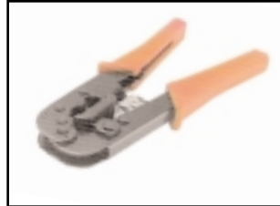
72-241 7.3" MODULAR CRIMP TOOL Cuts, strips, and crimps two types of plugs 6P & 8P in one. For crimping: 8P8C/RJ45, 6P6C/RJ12, 6P4C/RJ11 and 6P2C plugs. Steel body with easy grip plastic handles.
