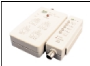
72-248 LAN & VOICE CABLE TESTER Tests for RJ45 modular connection with 258A, 568A & B, 356A wiring and 10 baseT & BNC coaxial. Includes 2 adapters for USOC RJ12 and RJ11 test usage. Performs test of cable continuity, miss wiring and polarization by the color of the L.E.D. indicators. Detachable remote unit for installed cabling. Powered using a 9V battery. Includes black ballistic nylon carrying case.
