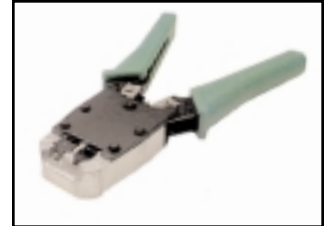
72-242 7.6" PRO MODULAR CRIMP TOOL For crimping 6P-RJ11 / RJ12 & 8P-RJ45, suitable for both stranded and solid wire. Provides precision crimping, cutting and stripping wire in one operation. Ratchet style mechanism.
