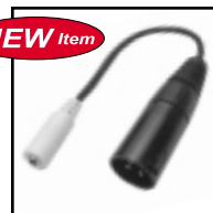
35-468 3.5mm stereo female jack to XLR male. Wired pin 1 = ground, pin 2 = tip & ring. 8" long. Black PVC jacket.
