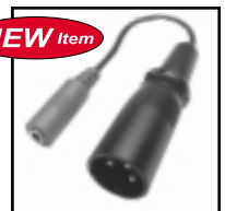
35-469 3.5mm stereo female jack to XLR male plug. Wired pin 1 = ground, pin 2 = tip, pin 3 = ring. 8" long. Black PVC jacket.
