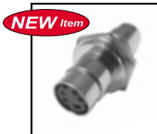
NEW Item 35-498BH (Nickel) 35-498G-BH (Gold) Bulkhead SVHS connector with flange. Panel mount 4 pin SVHS female to female. Mounts in 1/2" single "D" hole.
