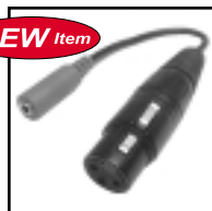
35-467 3.5mm stereo female jack to XLR female plug. Wired pin 1 = ground, pin 2 = tip, pin 3 = ring. 8" long. Black PVC jacket.
