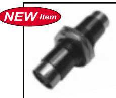
NEW Item 35-498 (Nickel) 35-498BC (Black chrome) Bulkhead SVHS connector with 2 nut mounting. Panel mount 4 pin SVHS female to female. Mounts in 1/2" double "D" hole.
