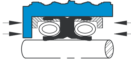
FIGURE 19. Bi-directional at Low Pressure
