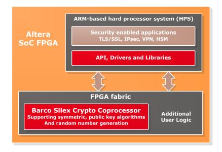
Figure 1 : Altera SoC FPGA with Barco Silex Cryptographic Coprocessor in FPGA and software drivers running on ARM processor
