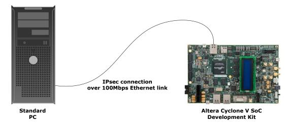
Figure 3 : Benchmark setup with IPsec connection between PC and SoC FPGA
