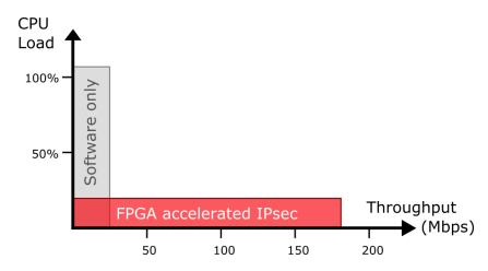
Figure 4 : Throughput and CPU usage comparison between software implementation and FPGA acceleration.
