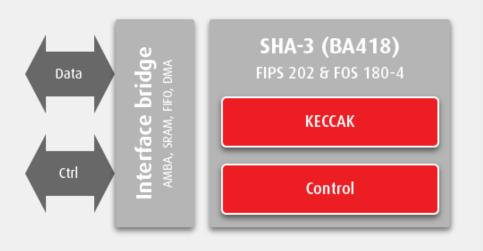
The SHA-3 core has integrated flexibility and scalability to allow for high throughput and a configurable number of hashing rounds to optimize the silicon resource/performance ratio.
