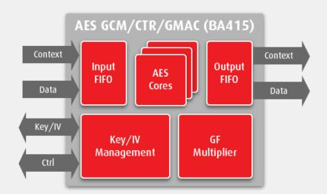
Figure 1: High-speed AES-GCM/CTR/GMAC block diagram
