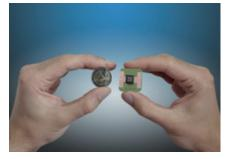
The sensing head with its dimensions of 28 x 28 millimeters is barely larger than a silver dollar.
