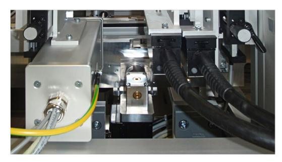
The high-performance printing system and camera unit is the heart of PALC. It can be attached to each side of the conveyor and can be adjusted to package size in both height and distance. A specialized IP 54 housing protects the camera and lens from soiling. Photo: ISW
