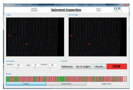
The application HMI of the spinning-plate capillary inspection system shows a live image of the current exposure on the left image section and a stored exposure of the reached angle position on the right. The current cursor position can be called up in a zoomed section for a more precise inspection. After an inspection run, the discovered faults, related to a 360° scale, can be displayed in the lower image section. Picture: ISW GmbH
