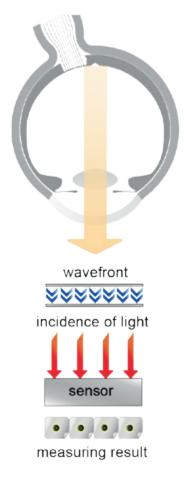
In wavefront analysis the generated pixels (black dots) are compared with the reference points of an ideal imaging lens (yellow points).
