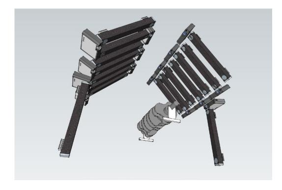
The image processingbased system comprises 16 carbon-fiber arms, each one holding two VGA Baumer cameras and a LED video projector. The system can be flexibly adapted to the size or complexity of a crankshaft. Photo: VIDEOMETRIC
