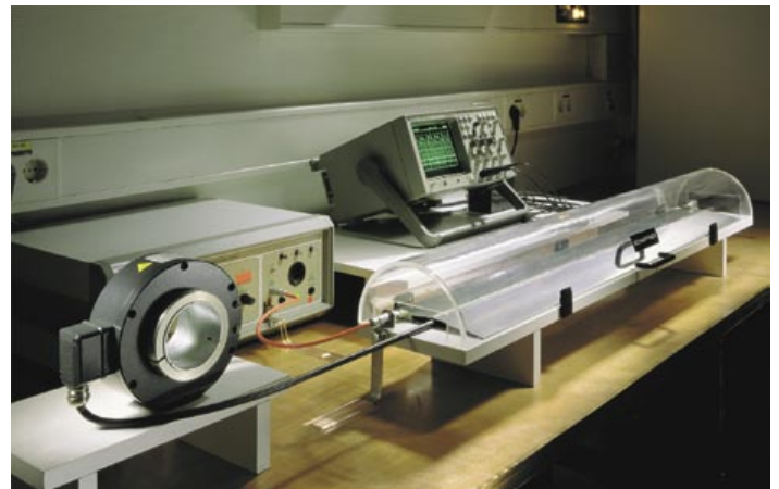
Fig. 4: In a test rig the electromagnetic compatibility (EMC) is optimized
