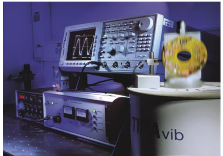
Fig. 3: Assembled PCBs are tested for resonant frequencies
