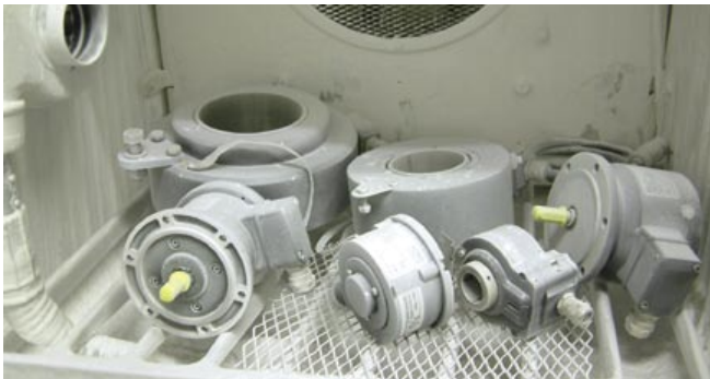
Fig. 6: The encoders are exposed to quartz dust blown into the dust-testing chamber
