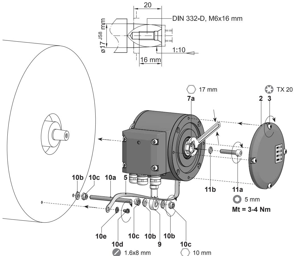
The encoder must be mounted with cable connection facing downward and not exposed to water.
