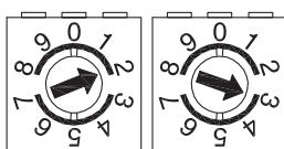
Address can be set by rotary switches. Example: User address 23
