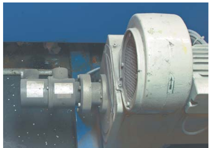
4: In spite of heavy dust pollution, the combination of a tachogenerator and centrifugal speed switch (TDP 0,2 + FSL) provides reliable operation on a web printing press
