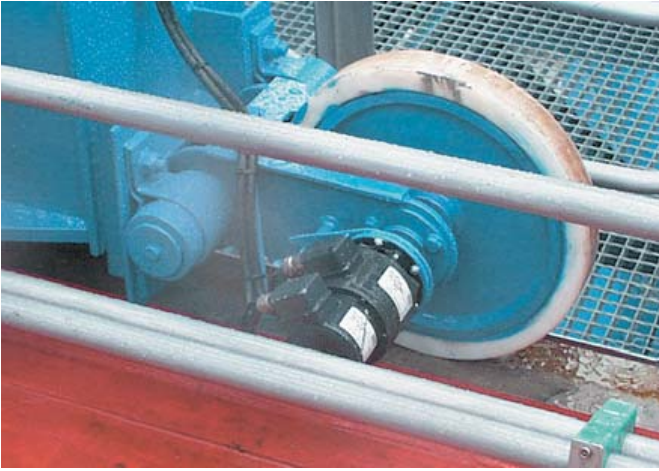
5: The POG 10G twin encoder, with a B10 Euro-flange and two separate sensor systems, fitted to the drive of a container crane
