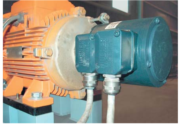
6: The twin hollow-shaft encoder HOG 10G is also fitted with two separate sensing systems
