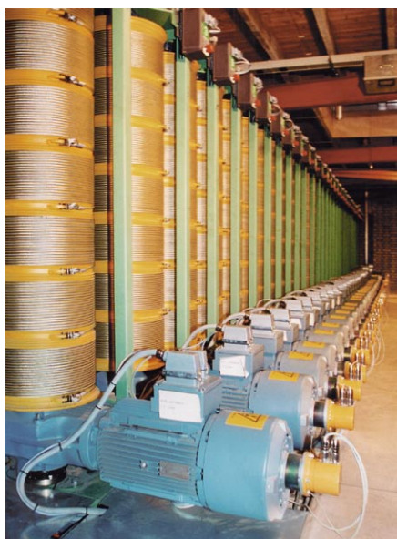
8: Absolute encoders on the drives of stage sets
