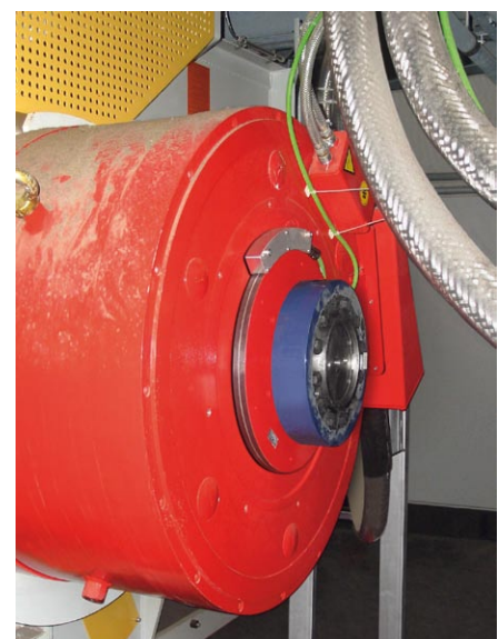
2: HeavyDuty absolute encoder on the torque motor in the shredder
