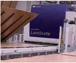
Inspection of flooring boards in the press line.
