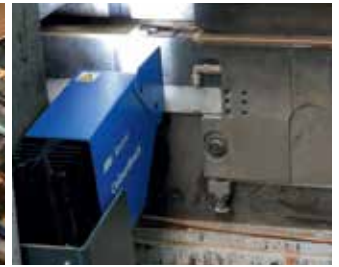
Automatic inspection of edge laquering.
