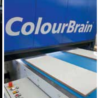
Inspection of high gloss furniture panels after lacquering.
