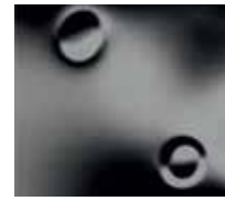
Fault in lacquering
