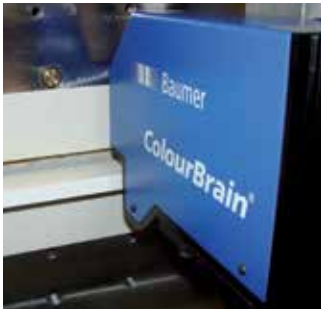
Inspection heads in the edge bander.
