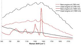
**Figure 1.** New (red lines) and used engine oil (black lines) characterized by 785 (dotted lines) and 1064 nm (solid lines) Raman spectroscopy. 785 nm laser excites high fluorescence from the samples which masks their Raman markers. Only 1064 nm produces high-quality Raman markers that clearly characterize the difference between new and used engine oils.
