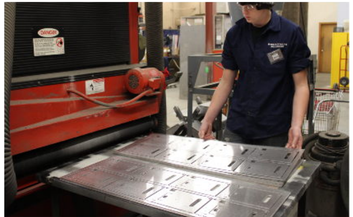
Turret presses punch and form full size sheet stock into component parts to precise shape and layout.
