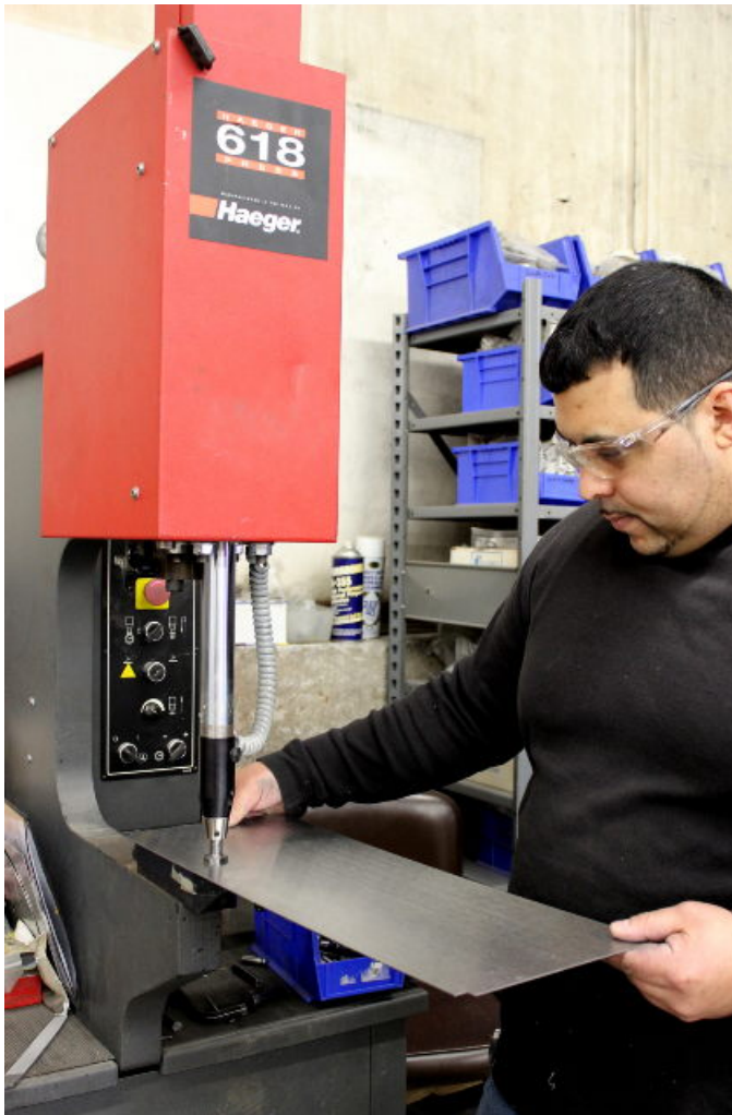
Fasteners are inserted and pressed into the components.
