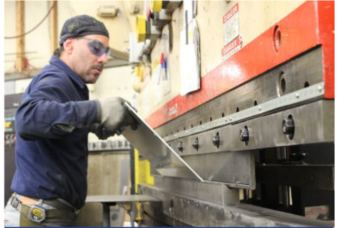
Metal is sheared, folded in hundreds of an inch tolerances by trained, highly skilled workers.
