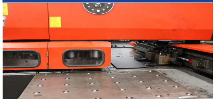
Turret presses punch and form full size sheet stock into component parts to precise shape and layout.
