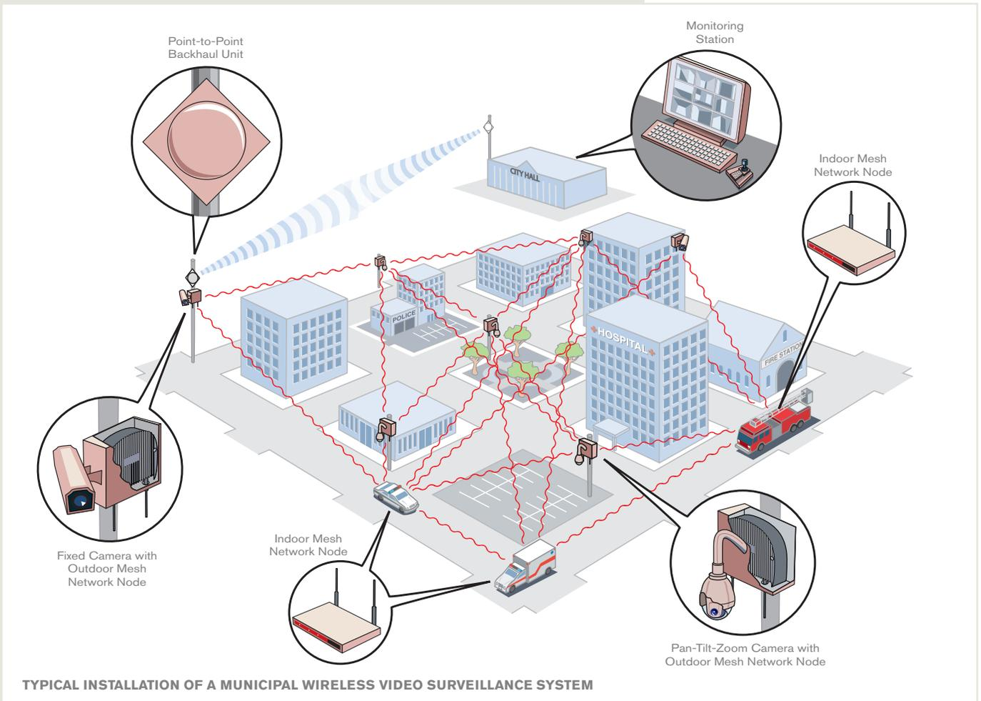
A mesh node, the piece of hardware that enables this mesh network system, is light enough to carry. A node can be placed in a mobile unit or trailer, it can be mounted on a roof or pole, or it can even set up as a command post. These nodes project the broadband IP connection to other nodes, sharing the connection with each other. Once the system is installed and activated, the nodes will find each other and create the wireless network.
