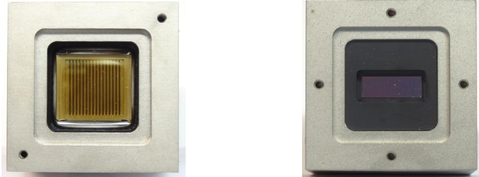
Fig. 41: Front face of the PML16C detectors (left) and of the PML-16 GaAsP detector (right)
