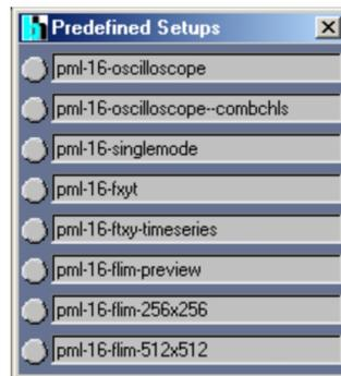
Fig. 26: Predefined-Setup panel. You can change between different instrument configurations by a single mouse click, see figure below.
