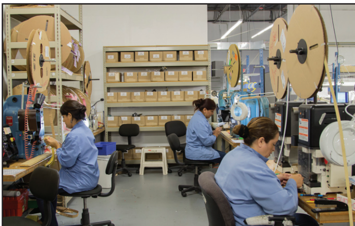
The most complex harness may have 100 wires and 50 connections, be up to 500 feet long and cost $12,000.
