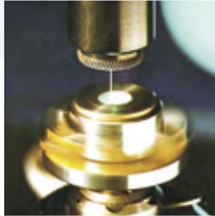
■ *Due to our long tradition of wire drawing, we have a comprehensive know-how in cold forming of metals. This is the basis of our wire drawing product range. Precise geometries and utmost durability are the attributes of our drawing dies. We offer a wide range of products made of carbide metal, diamonds and synthetic diamonds. Our PCD-tools reach dururances of up to a hundredfold compared to standard designs. This is a convincing reason for all our customers.*
