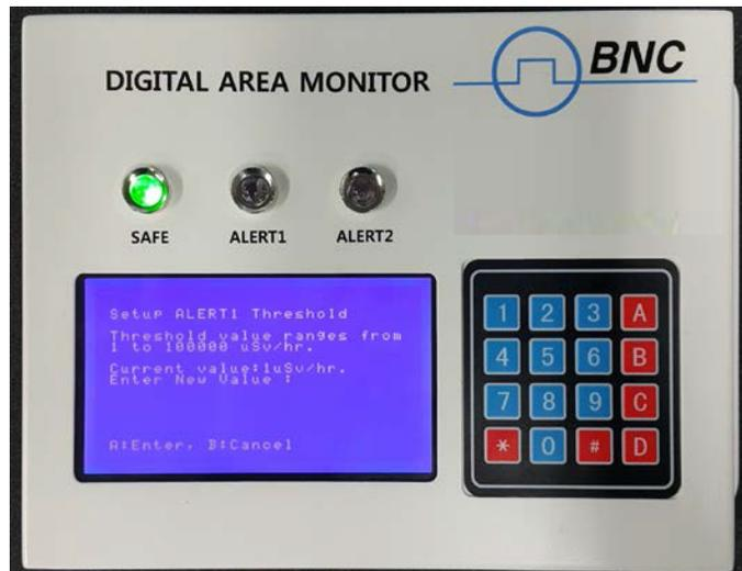
Figure 10. setup alarm threshold example (ALERT1 case)
