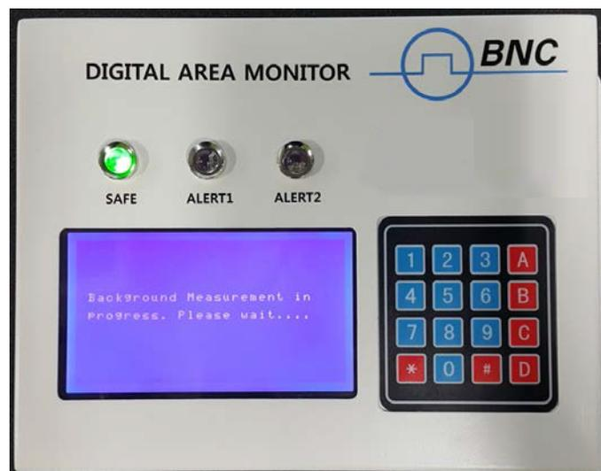
Figure 5. BNC™ MODEL 960 turn on message. Background measurement procedure
