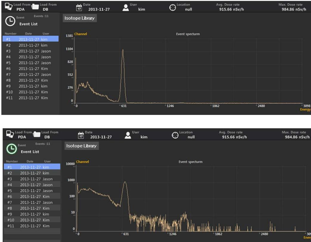
Figure 6.4 spectrum display change between linear and logarithm scale
