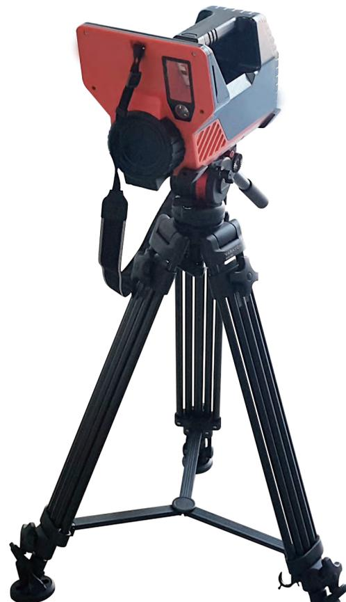
Tripod Mount for Radiation Detection
