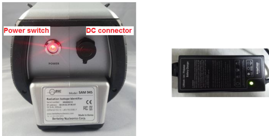
Figure 3.7. Detector unit (rear view) and AC adapter/charger
