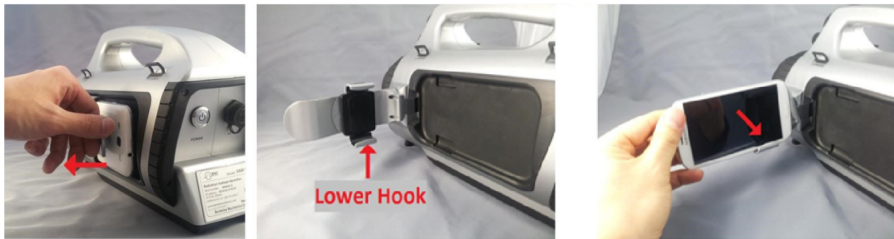
Figure 3.3. Attaching the smartphone to the detector
