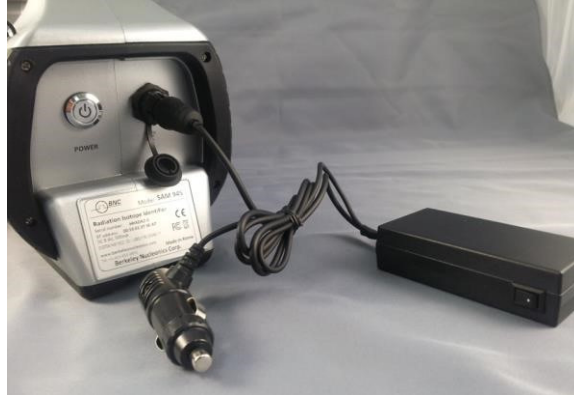
Figure 3.8. Detector unit (rear view) and vehicle adapter/charger
