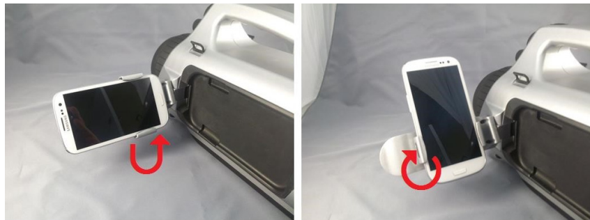
Figure 3.4. Tilting and rotating the smartphone holder
